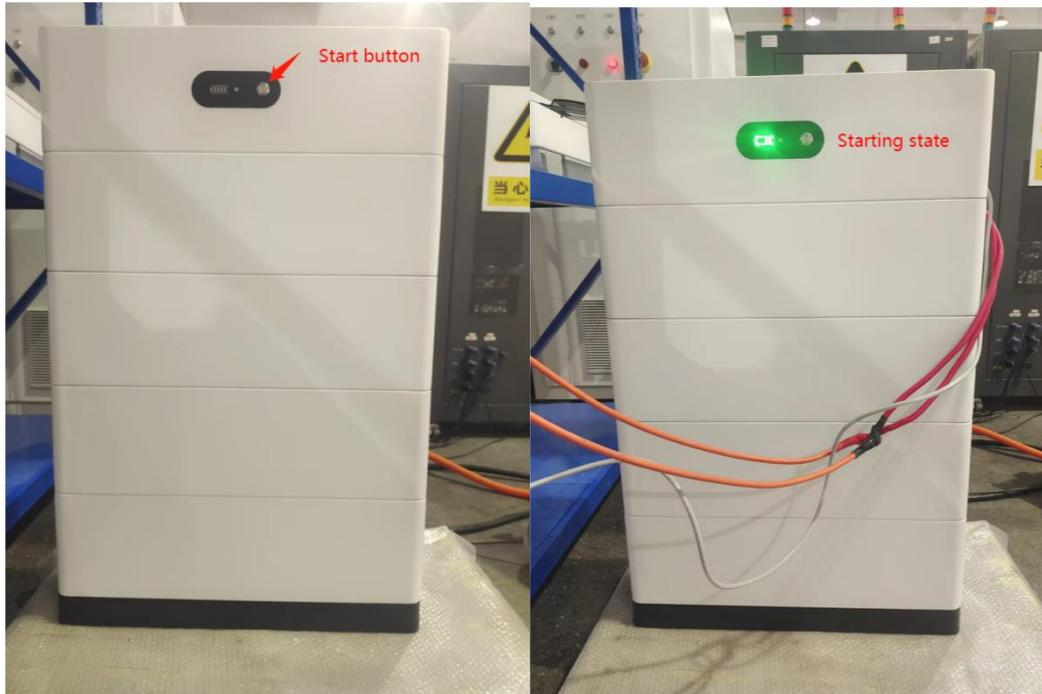
If the power grid does not supply power to the inverter, the high voltage output will wake up the inverter after the battery starts, and the inverter will communicate with the battery system by itself. After the communication is normal, the inverter screen will automatically display the battery information.
