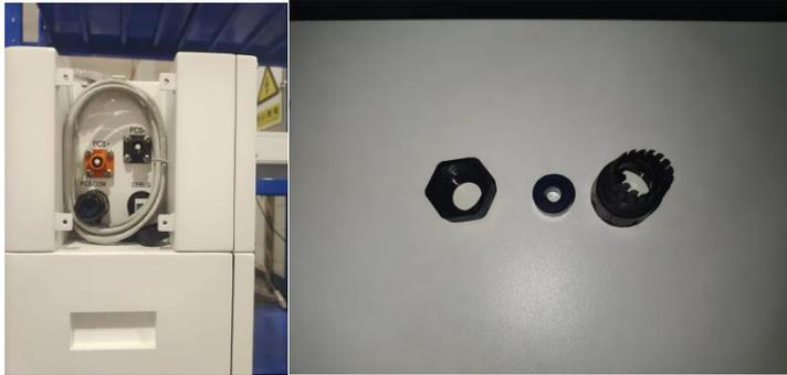
3. Assemble the waterproof pair connector with one end of the communication cable in the sequence shown in the following figure and tighten it. After connecting to the PCS COM port, tighten the pair connector (you can directly insert the network cable without connecting the waterproof head during indoor wiring). Connect the other end of the network cable to the inverter port terminal 7/8 with the blue/white blue pin
