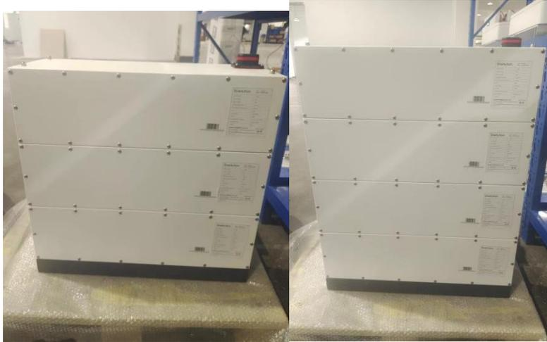
3. After batteries are stacked, check whether there is a gap between containers. If there is a gap, press the gap to ensure that the high voltage connection is normal.
