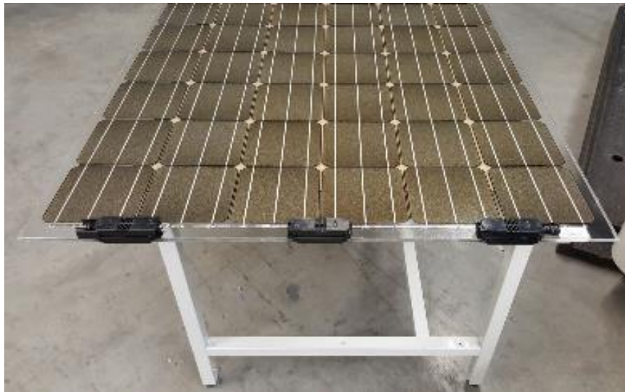
Image 2: rear side view of the j-box area. Clearly the the 3 pcs of j-boxes can be seen.
