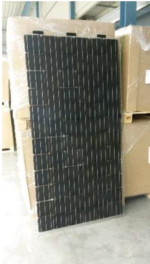
Image 1 (left): full view. The 72 pcs. of solar cells look dark blue/black from the front.
